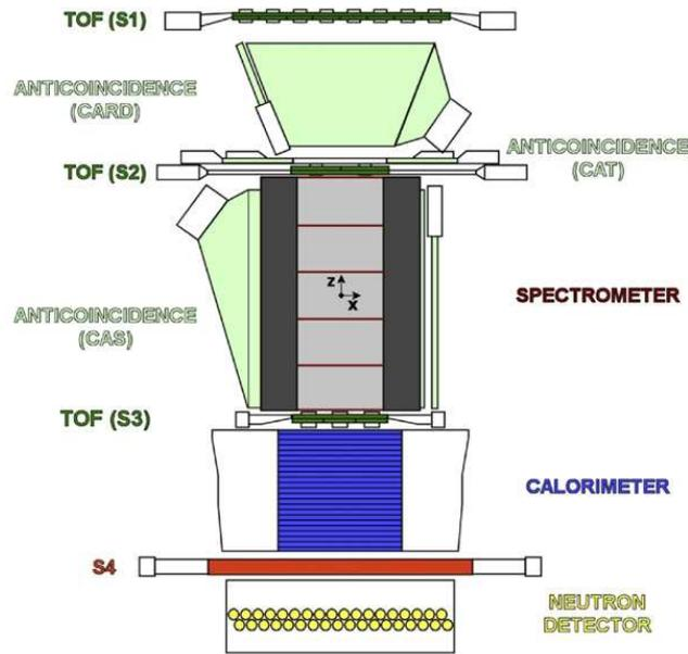
**Figure 1:** Schematic drawing of the Pamela apparatus.
